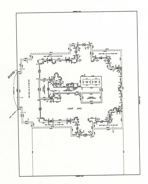
HORIZONTAL PLANES SHOWN HEREON ARE MEASURED FROM TOP OF FINISHED FLOOR TO BOTTOM OF FINISHED CELLING.
