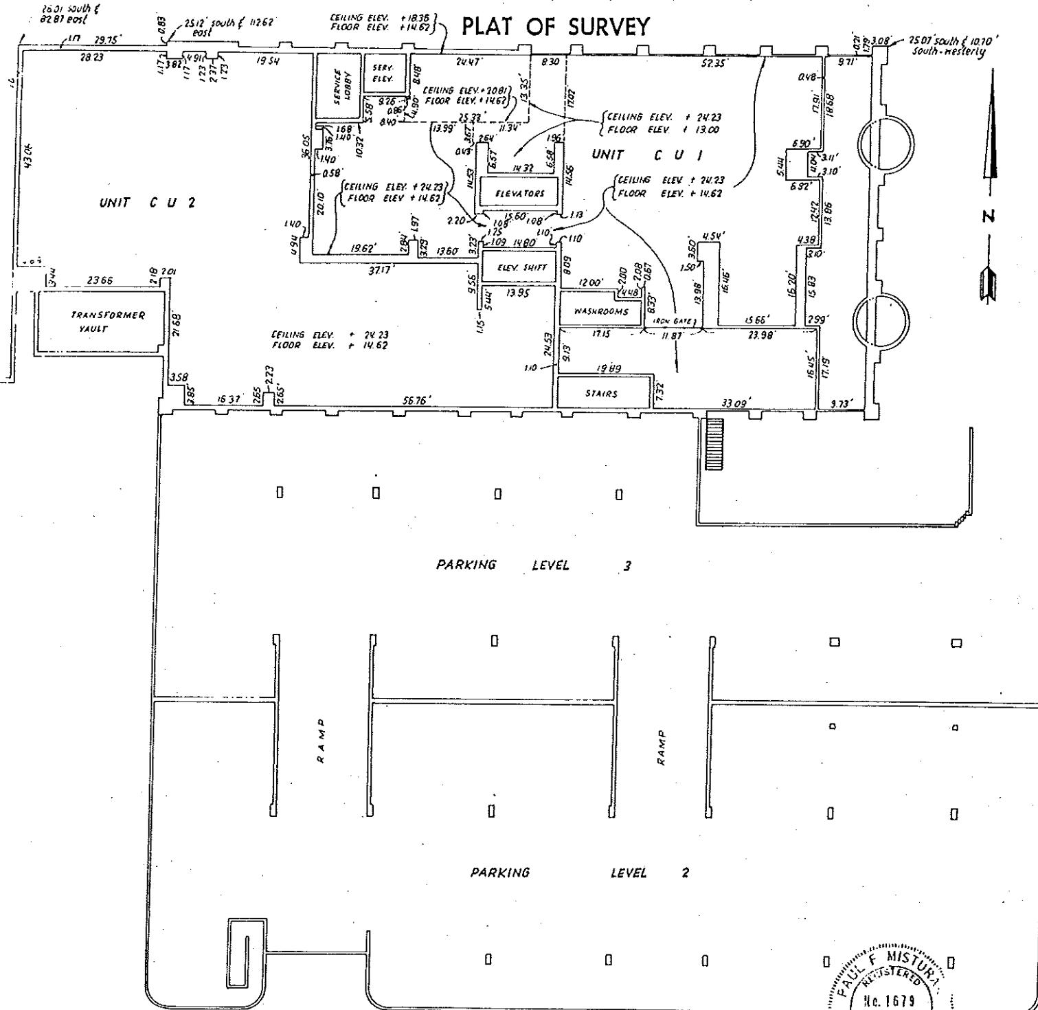
HORIZONTAL PLANES SHOWN HEREON ARE MEASURED ON THE TOP OF FINISHED FLOOR AND TO THE BOTTOM OF FINISHED CEILING.
